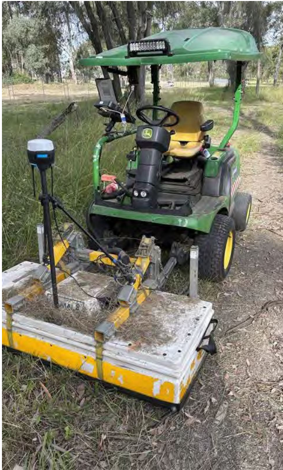
Figure 5: MALA MIRA 400MHz 3D GPR with RTK GPS mobilised with a John Deere Hydraulic Vehicle, used on site.
